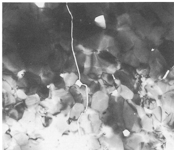
Figure 7 TEM observation of deformed (D) B composite: general view showing cracks and holes.
